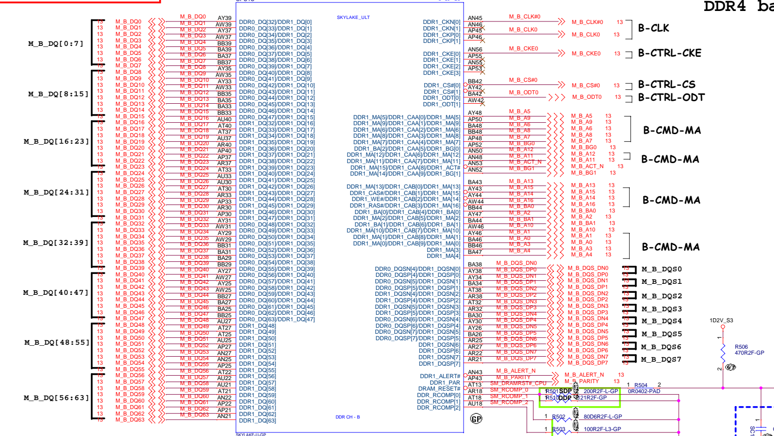
Figure 5-14. SKL U DDR4 6L Mixed SO-DIMM and Memory Down x16, T-Daisy Topology Memory Down Strobe/Data/Reset/RCOMP Signal Topologies
